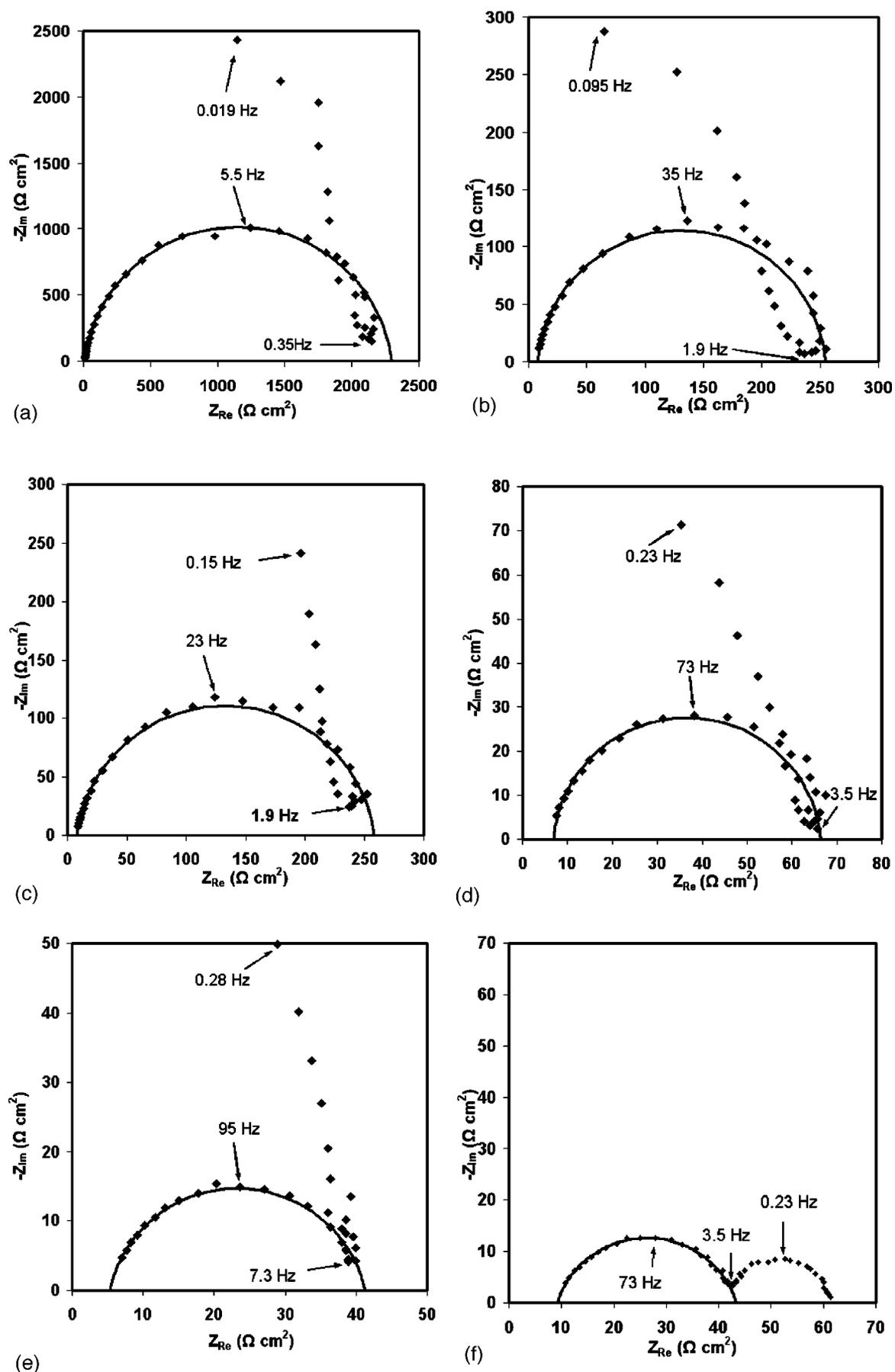
**Figure 4.** Nyquist representations for the impedance spectra ranging from  $10^{-2}$  Hz to  $10^3$  Hz in 2.5 M HF at (a, top left) 200, (b, top right) 50, (c, center left) -100, (d, center right) -250, (e, bottom left) -400, (f, bottom right) -550 mV vs. SCE.
