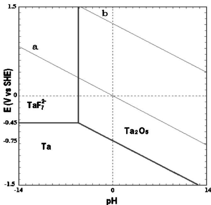
Figure 2. Pourbaix diagram for Ta in 1.0 M HF.
