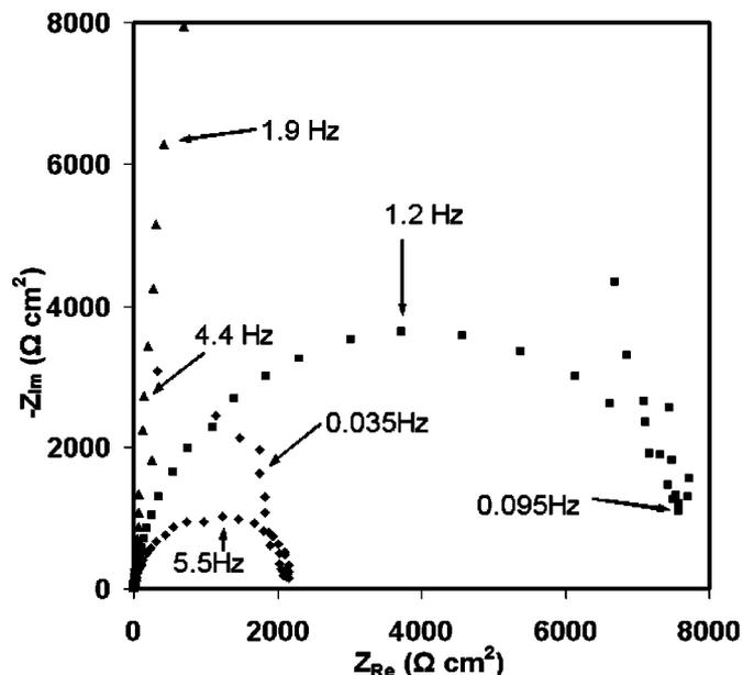
Figure 3. Nyquist representations for the impedance spectra ranging from  $10^{-2}$  to  $10^3$  Hz at +200 mV in (a) 2.5 M HF (♦), (b) 1.25 M HF/1.25 M  $\text{NH}_4\text{F}$  (■), and (c) 2.5 M  $\text{NH}_4\text{F}$  (●).
